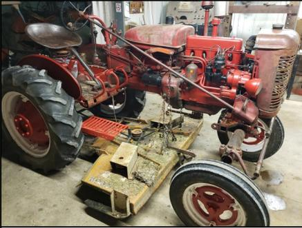
The Farmall Super A is finally outfitted with the Woods mower with all the hydraulics working, belts, pulleys.
